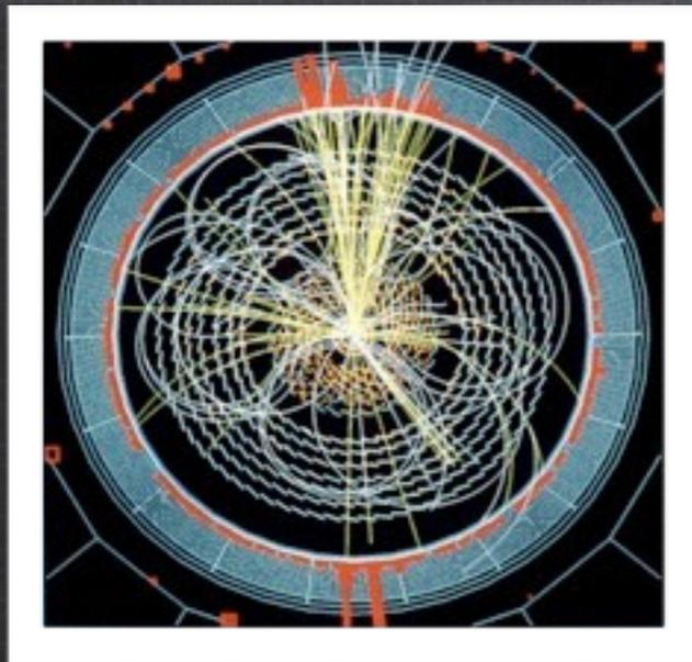
The detector can measure the decay products. The Higgs mass can be “reconstructed” using the measured energy and momentum of the particles.
